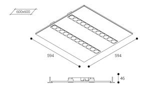
Installation: Keep a minimum 50 mm security distance between the luminaire and the ceiling to ensure its correct performance.
